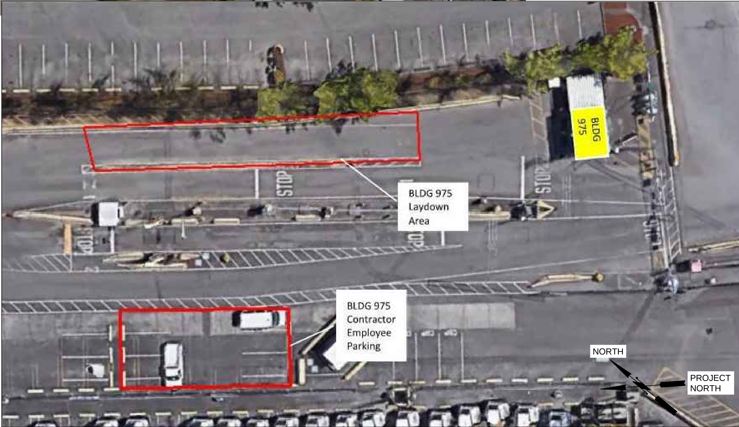
CONSTRUCTION STAGING AREAS - GUARDHOUSE 975
