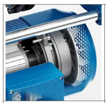
HOIST BRAKE: DEMAGS DC disk brake is a fail-safe type, electrically released, spring set for close positioning and motor start-up monitoring, with a minimum brake safety factor of 1.8. The brake is fast acting brake due to integrated electronic modules. The hoist (DMR) includes a brake sensor that monitors brake wear and will provide a warning to the operator if a brake adjustment is necessary. The high quality brake is designed for a minimum of 5 years life under single shift operation.
