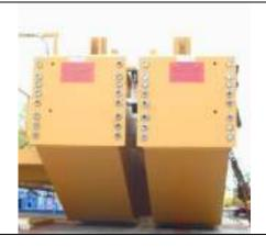
**GIRDER CONNECTION:** Feature: End trucks are bolted to girder ends to form a rigid connection. Bolts in shear or welded connections are not used.
