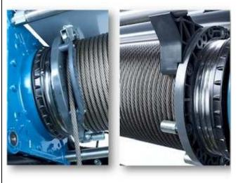
ROPE DRUM: Feature: Drum is of welded steel construction, with machined groove, optimized to a minimum depth of 0.375 times the rope diameter. Supported at each end by sealed anti-friction bearings, the drum is driven by a central splined shaft. To assure positive winding of rope on the drum and to prevent rope overlapping and potentially dangerous groove peak contact, a hoisting rope guide is employed.
