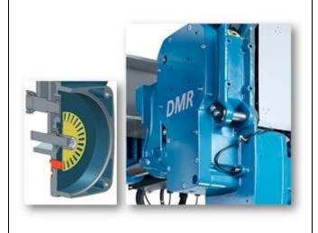
HOIST GEARING: Feature: All gear stages have helical gearing and are case hardened for low noises and smooth running. Each gear and hub connection is designed with a conical bonded press-fit connection. This means high resistance to vibration and insensitivity against load peaks. Gear lubricant is synthetic and does not require replacement for the normal life of the hoist. The standard hoist design is rated for FEM2m+ (20% greater duty than FEM2).
