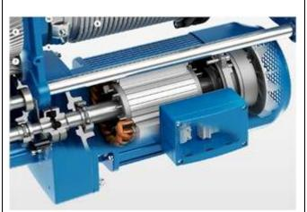
HOIST MOTOR: Feature: DEMAG designed and manufactured, these motors offer dependable performance with a minimum of maintenance. An optimized motor design for low-vibration, quiet operation 12/2-pole squirrel-cage motor with cylindrical rotor. All motors have Class F insulation and are protected from overheating by thermal protectors imbedded in the windings. Motors are totally enclosed, fan cooled (TEFC). Enclosure is outdoor rated IP 55 with a duty of 60% running time and 360 starts/hour.
