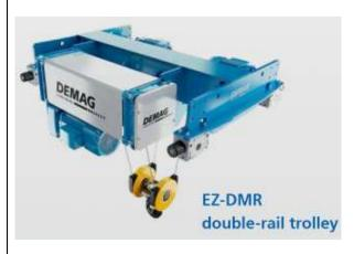
**TROLLEY:** Feature: The EZDMR close headroom double rail trolley supports the hoist on one side of the beam allowing an excellent high-hook dimension. The precision machined and welded steel trolley frame includes drops stops and lifting lugs for transport and installation. The compact design allows for minimum hook approach dimensions.
