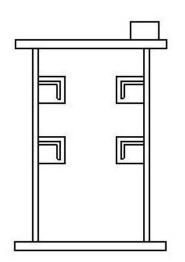
**GIRDERS:** Feature: Girders for double girder cranes are fabricated plate box sections, with diaphragms, designed to resist all vertical horizontal, and torsional forces. Trolley rails are ST52 rectangular sections welded directly over girder webs, to optimize transmission of loads into the girder structure.
