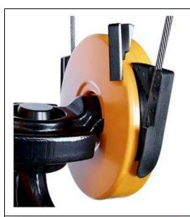
BOTTOM BLOCK: Feature: Bottom block has a totally enclosed housing fabricated of steel. The rope sheaves are supported on anti-friction bearings and the hook is forged alloy-steel and supported on an anti-friction thrust bearing. Hook is equipped with a heavy spring safety latch. A handle recess makes it easier to be gripped and handled. Moving plastic elements close the opening where the rope enters and leaves the bottom block thus preventing the hands from getting caught and jammed.
