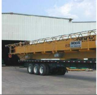
CRANE WALKWAY: Feature: Full length walkway fabricated from steel checkered safety plate with 4 inch high toe guards on all sides. The steel handrails are fabricated from 1 1/2 inch square tubing and are 42 inches high. The All Welded Construction allows the walkway to become an integral part of the box girder.
