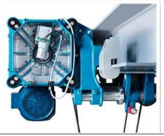
**LIMIT SWITCH:** Feature: Hoist is equipped with a 4 position geared upper and lower limit switch. This switch is easily adjusted to set the extreme upper and lower limits of hook travel. The limit switch is equipped with a digital drum revolution counter for use in evaluating service conditions and maintenance intervals.
